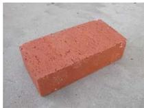
220x110x 55  | NF EN 771-1 | 4.7<br>(bending test)         |
